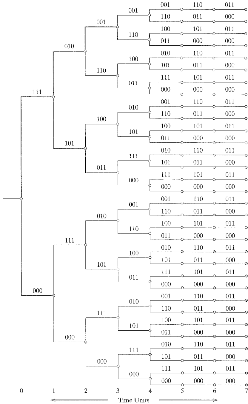
FIGURE 13.1: The code tree for a (3, 1, 2) encoder with h = 5 .
