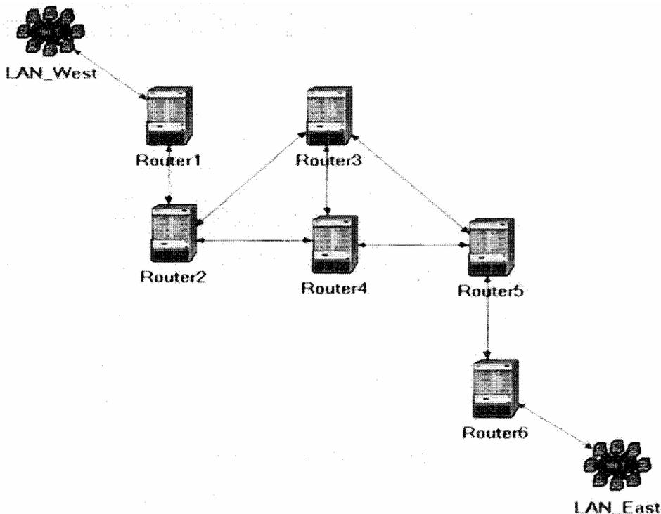
The **ethernet4\_slip8\_gtwy** node model represents an IP based gateway supporting four Ethernet hub interfaces and eight serial line interfaces. IP packets arriving on any interface are routed to the appropriate output interface based on their destination IP address.
