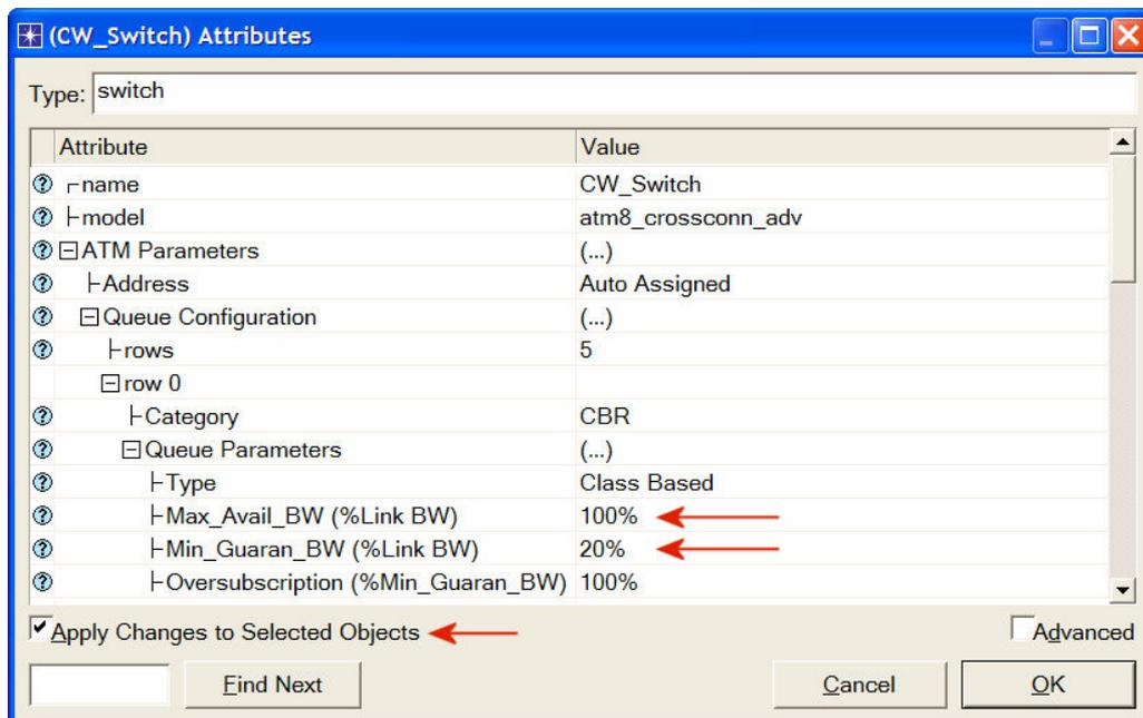
**Max\_Avail\_BW** is the maximum bandwidth allocated to this queue. Calls will be admitted into this queue only if they are within the maximum available bandwidth requirement.
