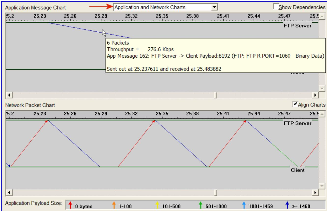
The Network Chart shows that this application message causes many packets to flow over the network. These packets are a mix of large (blue and green) packets from the FTP Server to the Client and small (red) packets from the Client to the FTP Server. As the red color indicates, these packets contain 0 bytes of application data. They are the acknowledgments sent by TCP.
