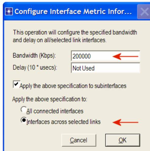
5. Repeat step 4 for all links with a cost of 10 but assign 100,000 Kbps to the **Bandwidth (Kbps)** field.
