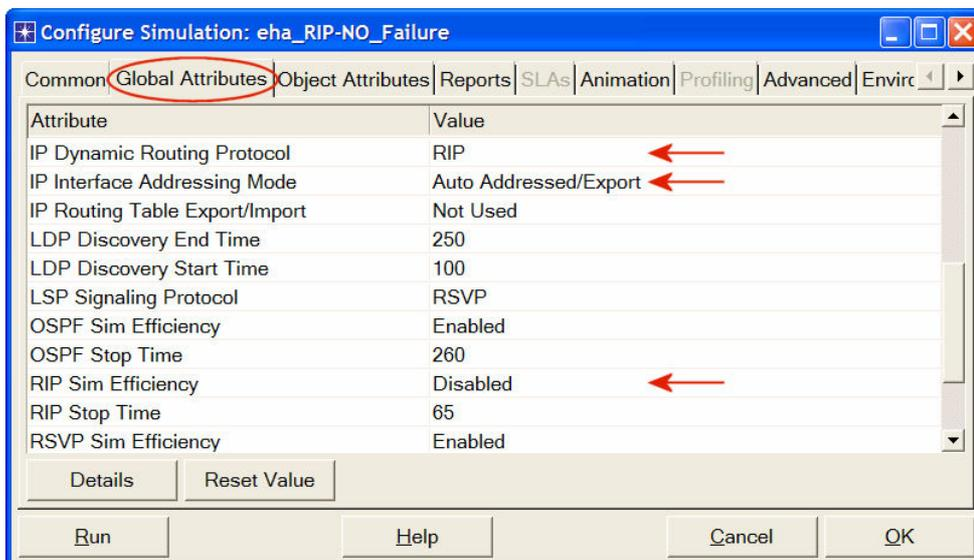
**Auto Addressed** means that all IP interfaces are assigned IP addresses automatically during simulations. The class of address (e.g., A, B, or C) is determined based on the number of hosts in the designed network. Subnet masks assigned to these interfaces are the default subnet masks for that class.
