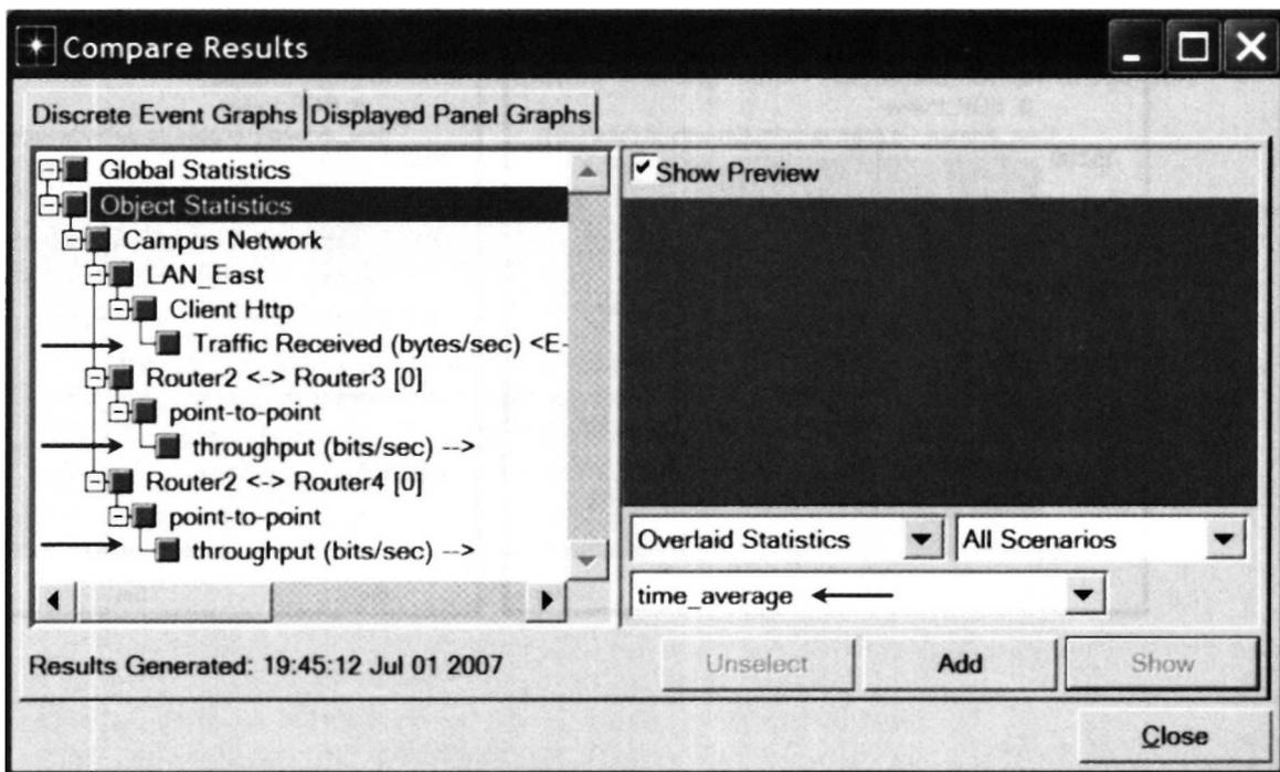
3. Select and show the graphs of the following statistics: **Traffic Received** in **LAN\_East**, **throughput** in the **Router2-Router3** link, and **throughput** in the **Router2-Router4** link. The resulting graphs should resemble the graphs below.
