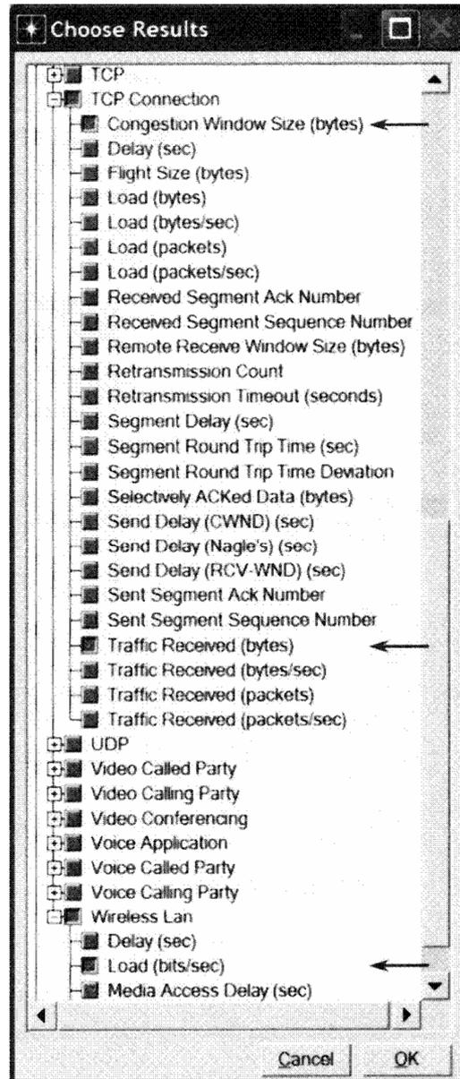
4. Right-click on the **Traffic Received (bytes)** statistic. ⇒ Choose **Change Collection Mode**. ⇒ In the dialog box check **Advanced**. ⇒ From the drop-down menu, assign **all values** to **Capture mode**.
