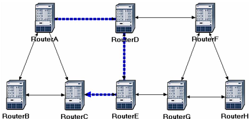
4. Repeat step 2 to show the route for the traffic demand between **RouterB** and **RouterH**. The route is as shown below. (Note: Depending on the order in which you created the network topology, the other “equal-cost” path can be used, that is, the *RouterB-RouterA-RouterD-RouterF-RouterH* path).
