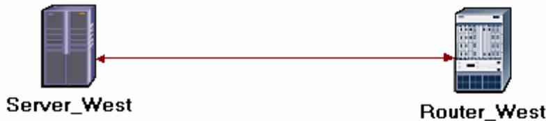
The **ethernet4\_slip8\_gtwy** mode model represents an IP-based gateway supporting four Ethernet hub interfaces and eight serial line interfaces.
