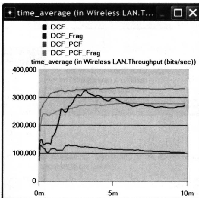
**Throughput** represents the total number of bits (in bits/sec) forwarded from wireless LAN layers to higher layers in all WLAN nodes of the network.
