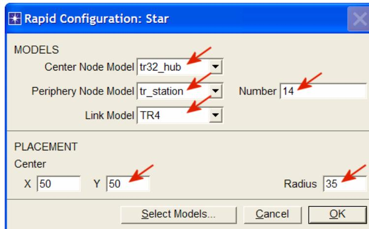
The **tr.32\_hub** node model is a token ring hub supporting up to 32 connections at 4 or 16 Mbps. The hub forwards an arriving packet to the next output port. There is no queuing of packets in the hub itself as the processing time is considered to be zero.
