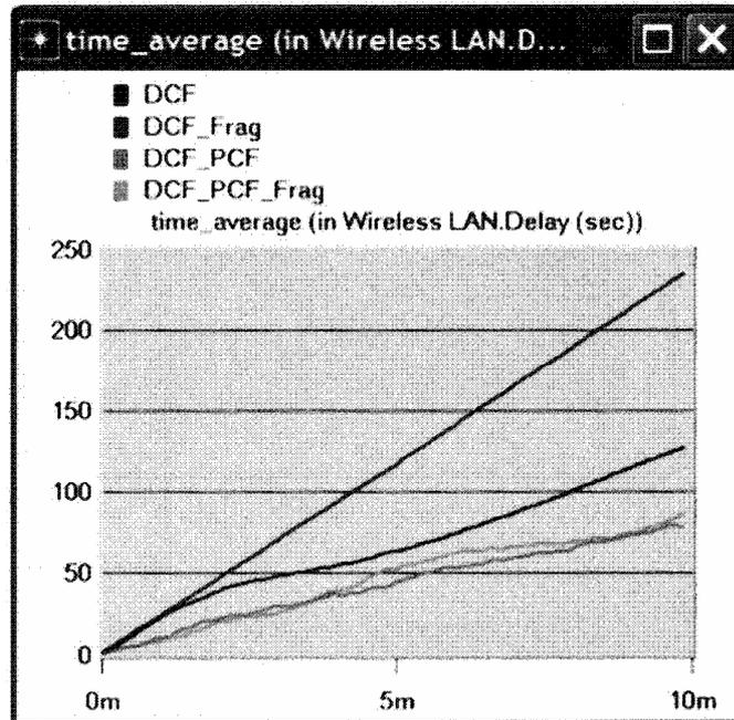
**Delay** represents the end-to-end delay of all the packets received by the wireless LAN MACs of all WLAN nodes in the network and forwarded to the higher layer. The delay includes medium access delay at the source MAC, reception of all the fragments individually, and transfer of the frames via AP, if access point functionality is enabled.
