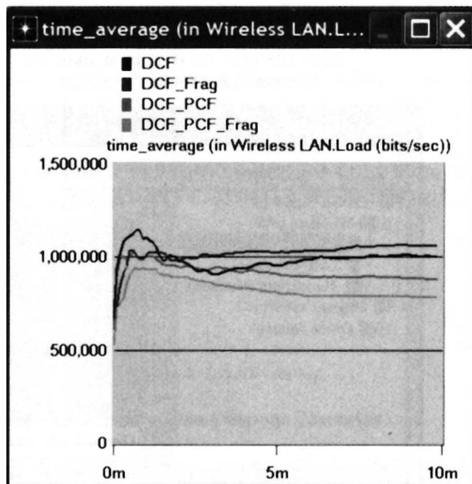
**Load** represents the total load (in bits/sec) submitted to wireless LAN layers by all other WLAN nodes of the network. The statistic does not include the bits of the higher layer packets that are dropped by WLAN MACs upon arrival and not considered for transmission due to, for example, insufficient space left on the higher layer packet buffer of the MAC.
