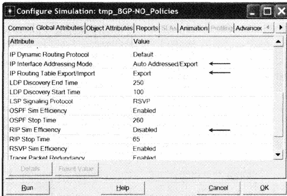
**Auto Addressed** means that all IP interfaces are assigned. IP addresses automatically during simulation. The class of address (e.g., A, B, or C) is determined based on the number of hosts in the designed network. Subnet masks assigned to these interfaces are the default subnet masks for that class.
