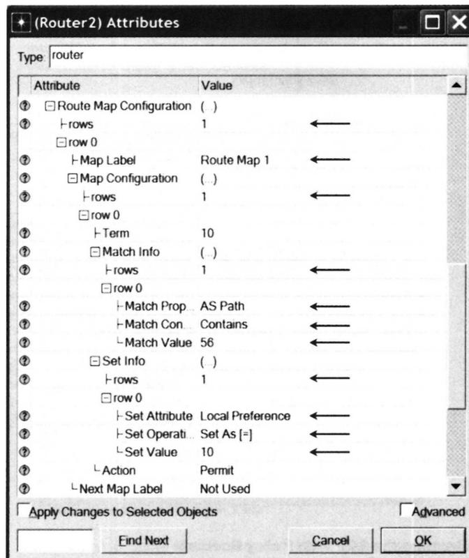
The next step is to assign the above route map to the link connecting **Router2** to **Router3**. This way traffic from **Router2** to AS 56 will be preferred to go through **Router4** instead.
