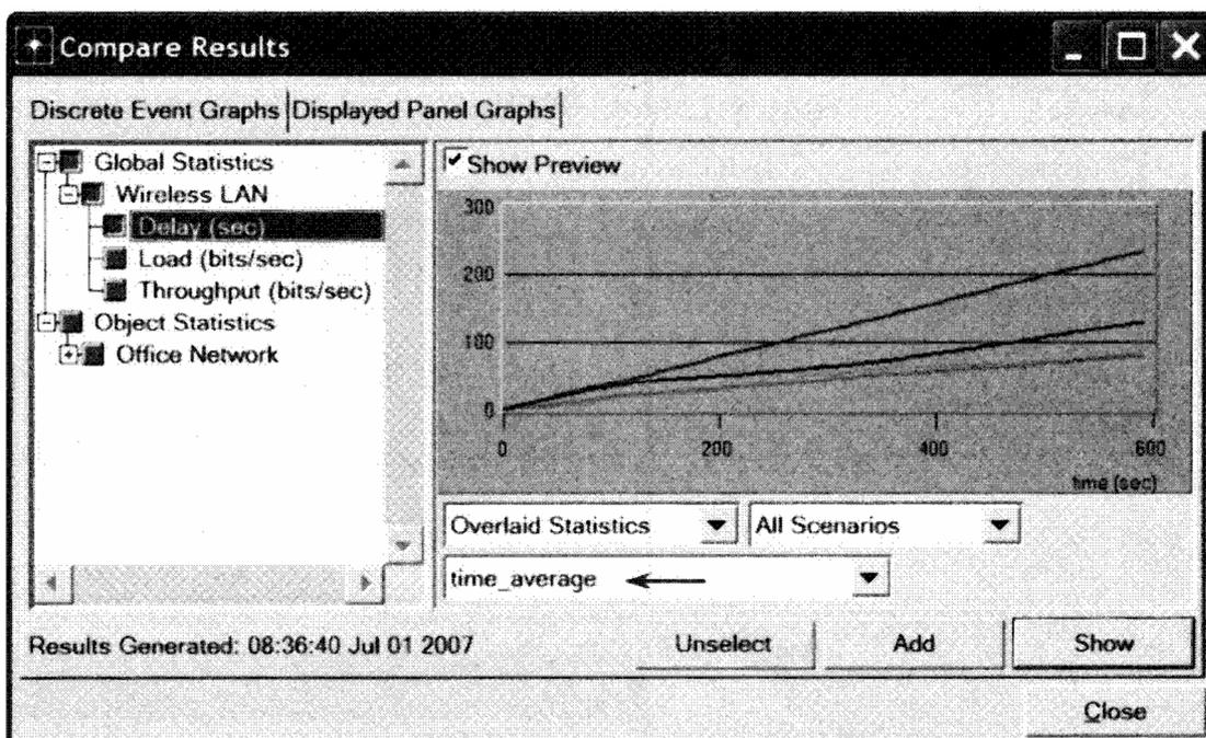
**time\_average** is the average value over time of the values generated during the collection window. This average is performed assuming a "sample and hold" behavior of the data set (i.e., each value is weighted by the amount of time separating it from the following update and the sum of all the weighted values is divided by the width of the collection window),
