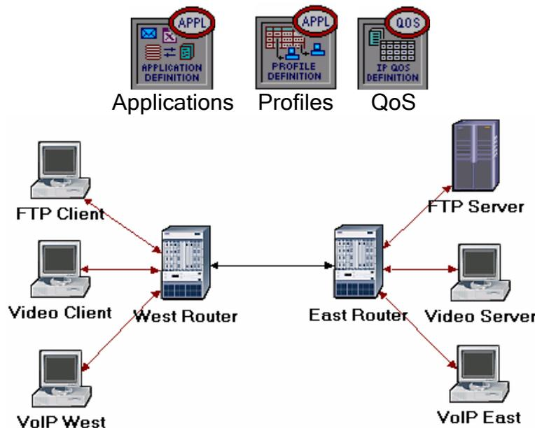
The **QoS Attribute Config** node defines attribute configuration details for protocols supported at the IP layer. These specifications can be referenced by the individual nodes using symbolic names. It defines different queuing profiles such as FIFO, WFQ, priority queuing, custom queuing, MWRR, MDRR, and DWRR.
