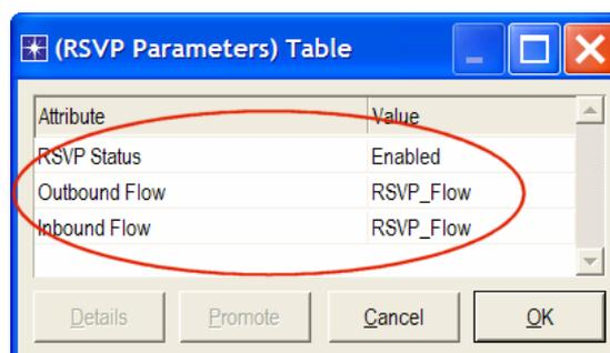
Note that the characteristics of the **Outbound Flow** are carried in the Path messages to be sent from sender to receiver, and the characteristics of the **Inbound Flow** parameters are carried in the Resv messages to be sent from the receiver to the sender.
