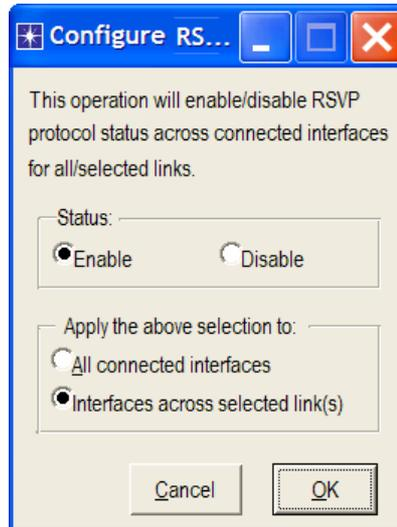
The above process enables RSVP on all interfaces along the path between the two Voice parties that need to utilize RSVP.
