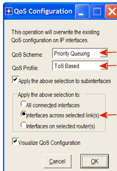
**Note:** Since the **Visualize QoS Configuration** radio button is checked, the link is colored based on the QoS scheme used (orange for priority queuing).
