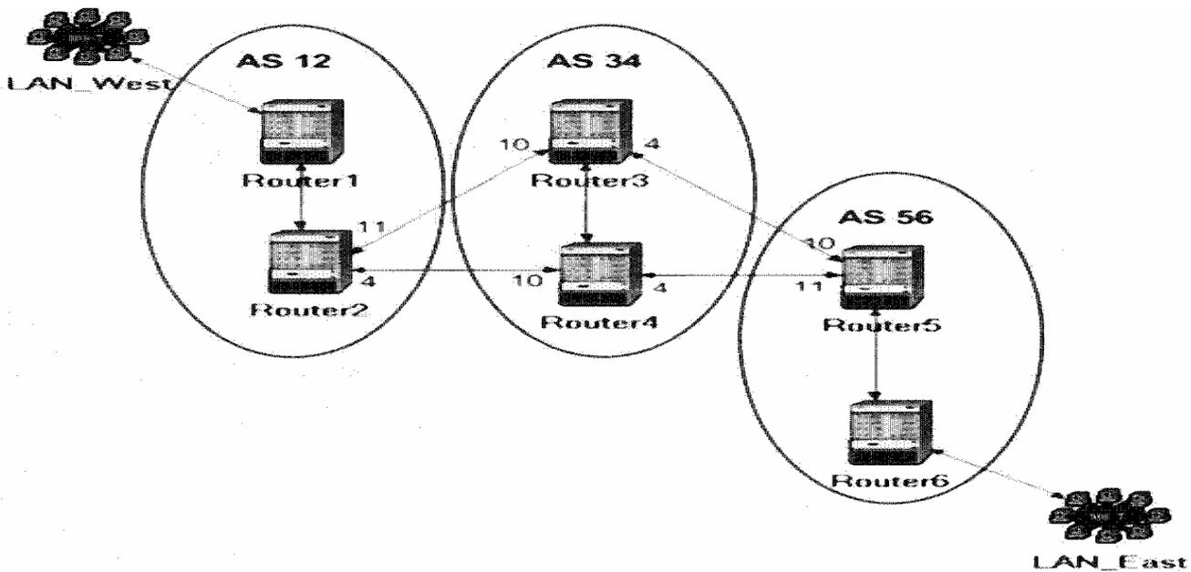
6. Right-click on **Router2** ⇒ **Edit Attributes** ⇒ Expand the **IP Routing Parameters** hierarchy ⇒ Expand the **Interface Information** hierarchy ⇒ Expand row 4 hierarchy. ⇒ Click on the values of the **Routing Protocol(s)** attribute ⇒ Disable **RIP** as shown ⇒ Click **OK** twice.
