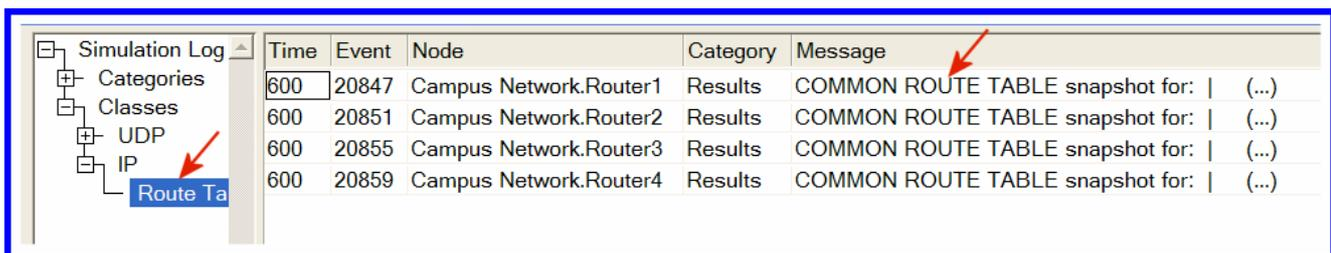
2. Carry out the previous step for the **Failure** and **NO\_Failure** scenarios. The following are partial contents of **Router1**'s routing table for both scenarios (Note: Your results may vary due to different nodes placement):
