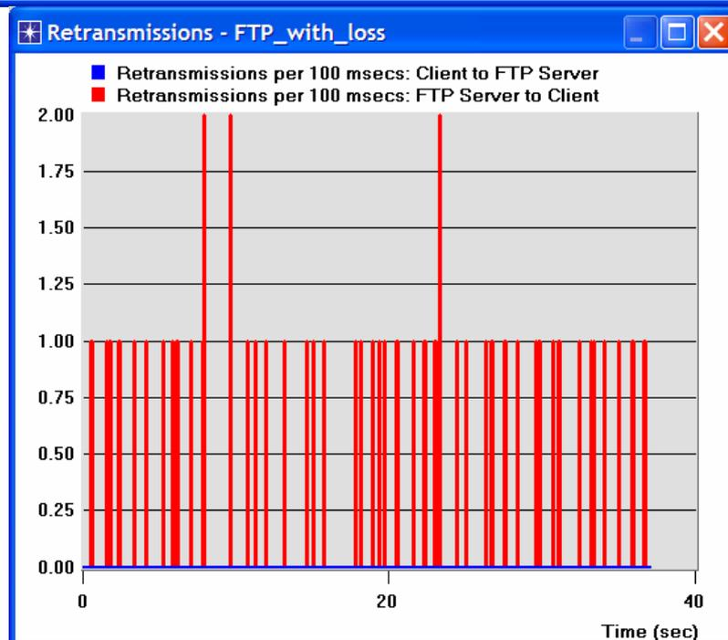
ACE divides the entire tasks duration into **buckets** of time and calculate a mean of total value for each interval. The default bucket width is 1000 msec; you can change this value in the Bucket Width (msec) field of the ACE statistic hardware.
