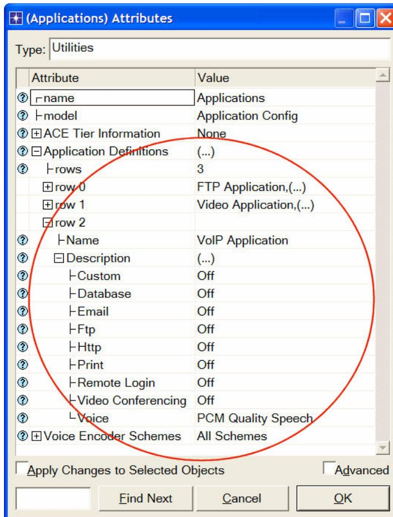
**Type of Service** (ToS) is assigned to the IP packets. It represents a session attribute that allows packets to be provided the appropriate service in the IP queues.
